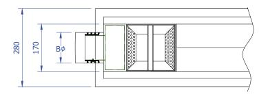
The blue measurements indicate the variable dimensions shown in the chart above. All dimensions in mm.
