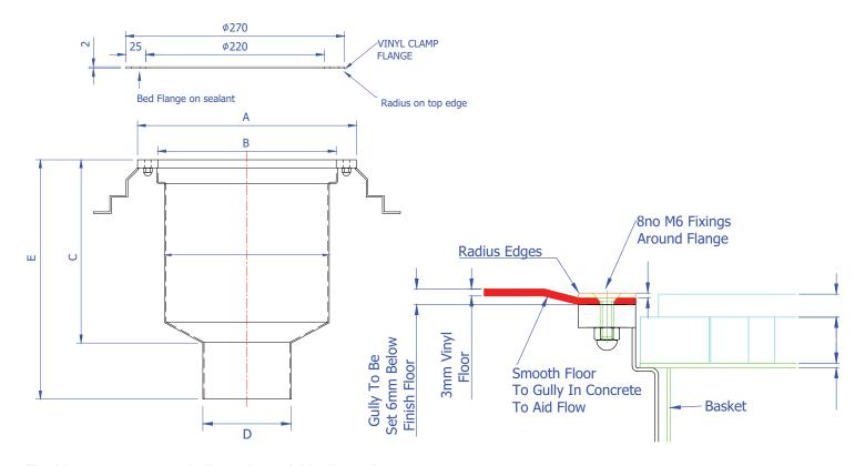
The blue measurements indicate the variable dimensions shown in the chart above. All dimensions in mm.
